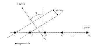
Fig. 3. Uniform Linear Array Structure
