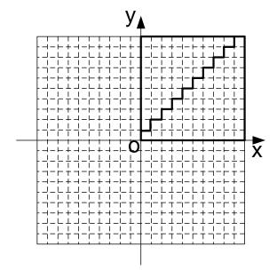
Fig. 1. Division of the unit cell of a 2D photonic crystal with square lattice. One of the unit cells has not the mirror symmetry with respect to the y=x plane and the other has the above mirror symmetry.
