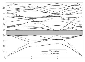
Fig. 2. (a) The best GaAs photonic crystal without mirror symmetry with respect to y=x plane. (b) The corresponding photonic band structures.
