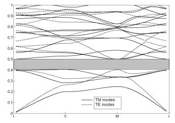
Fig. 3. (a) The best GaAs photonic crystal with mirror symmetry with respect to y=x plane. (b) The corresponding photonic band structures.
