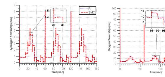
Fig 11.Mass flow rates of Hydrogen at anode and Oxygen at cathode
