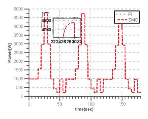
Fig 9.PEMFC power output
