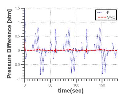
Fig13. Pressure difference between reactants at anode and cathode
