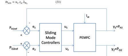
Fig 2. Proposed Sliding Mode Controllers for pressure regulation of PEMFC
