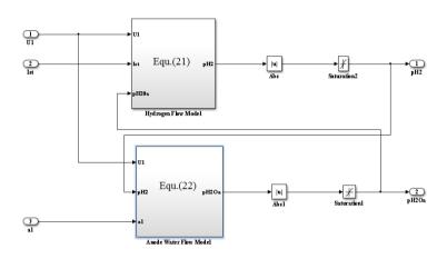
Fig 5. Anode Model
